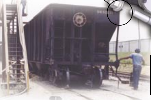
Simply twist nut to secure vibrator to bracket
